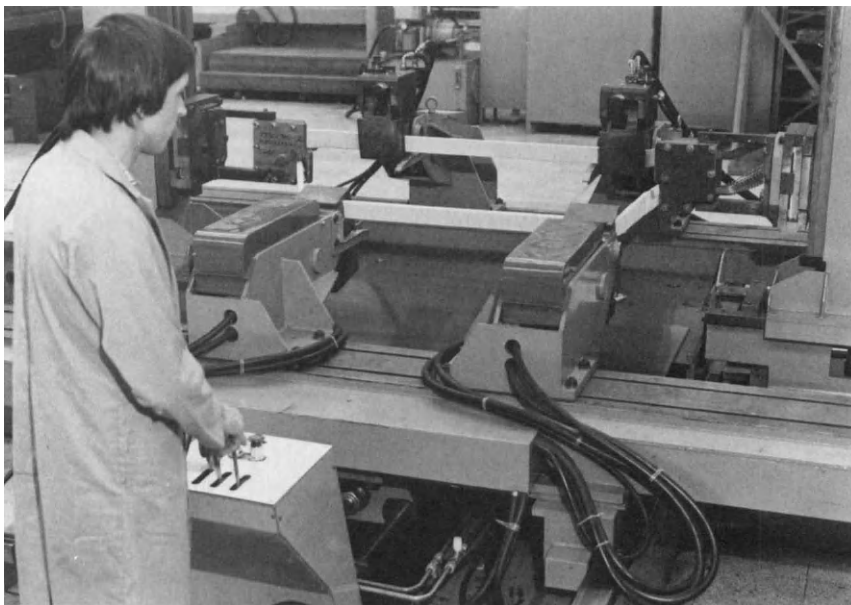
Figure 6.15 High-voltage stator coil – pulling out a diamond-shaped coil
