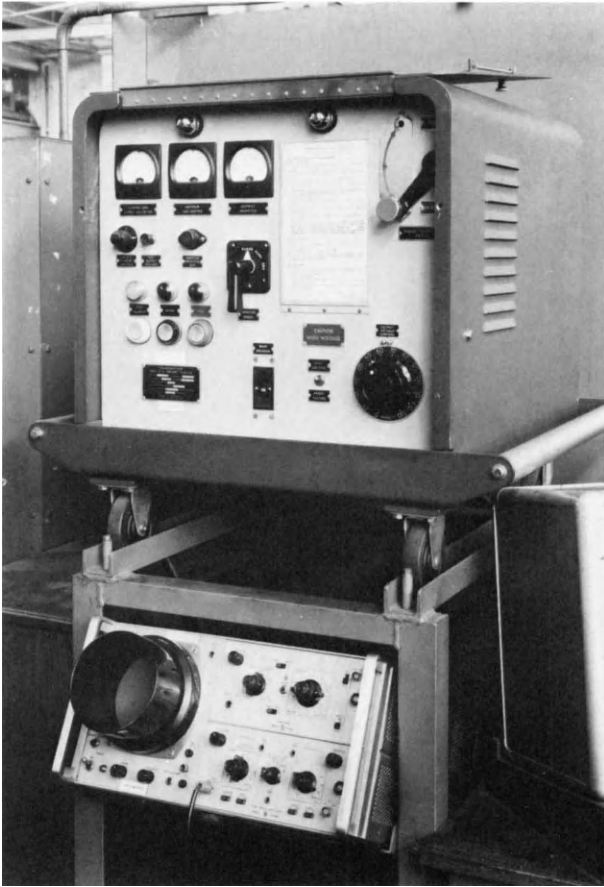
Figure 6.32 Surge tester (30 kV) for checking interturn insulation
