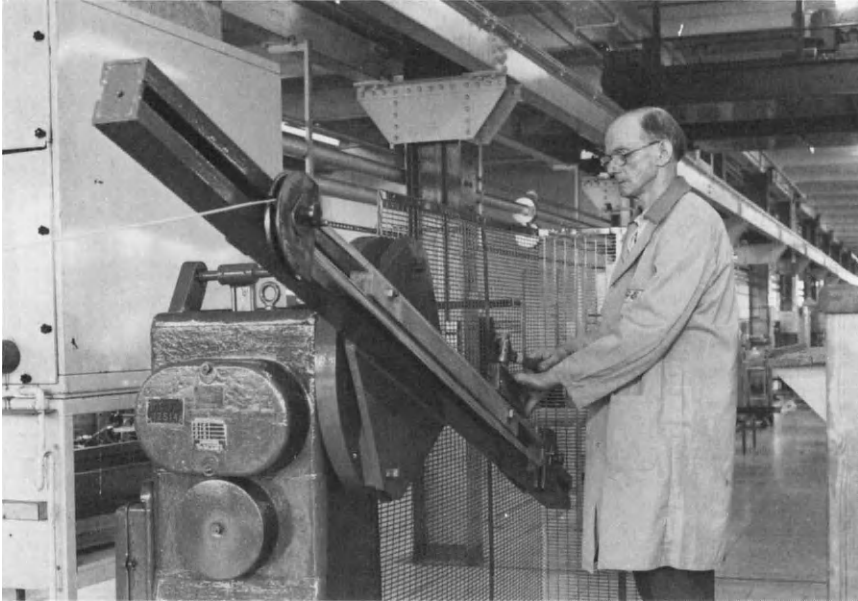
Figure 6.12 High-voltage stator coil – winding the coil loop
